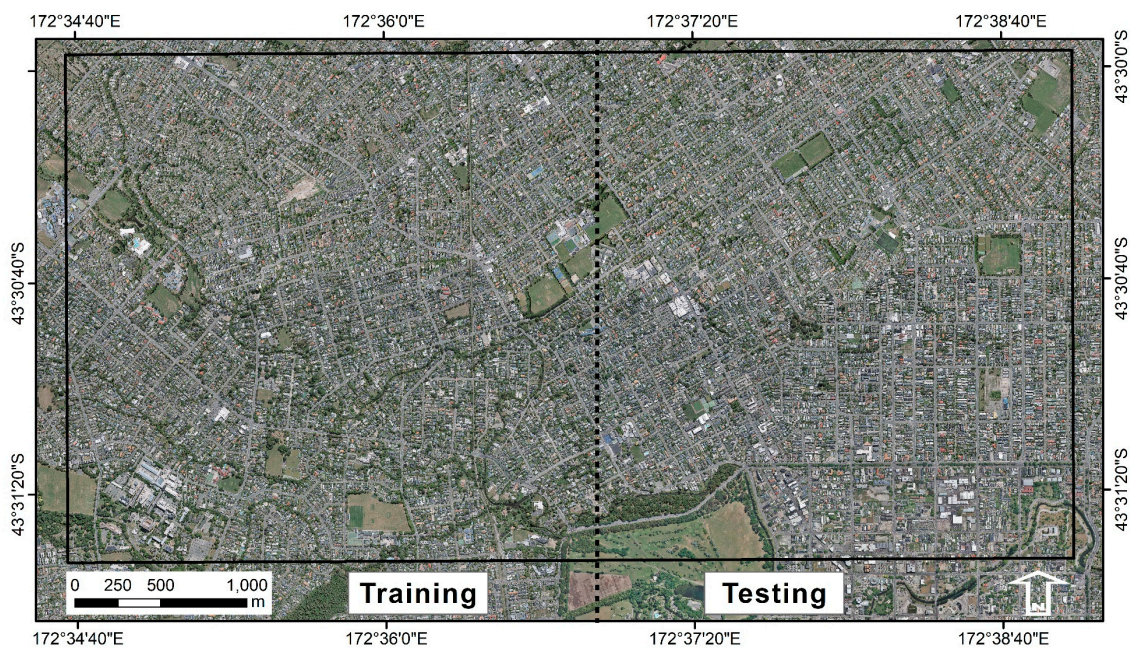
Figure 4. Overview of the dataset (an urban area of Christchurch City, New Zealand) used in the present study. The black dotted line separates the image into training and testing datasets for evaluating the performance of the proposed DeepResUnet by comparing it with other state-of-the-art deep learning approaches.
