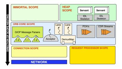
Figure 5: Scoped Zen Server Scoped Memory Architecture.
